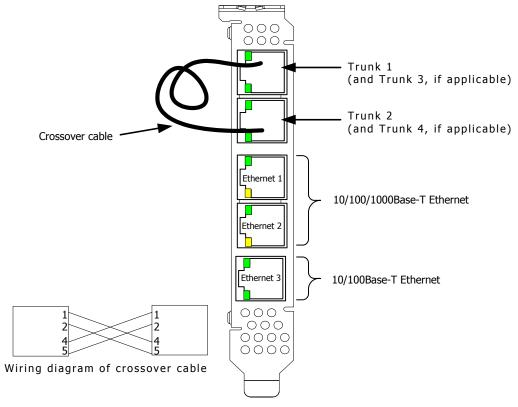
The crossover cable connects the transmit signals from one trunk to the receive signals on another trunk by connecting the pins as shown.
