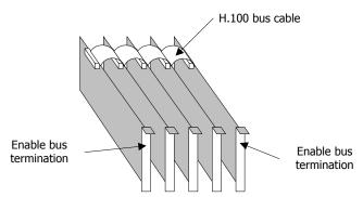
DIP switch S1 controls the H.100 bus termination. By default, all S1 switches are set to the OFF position (H.100 bus termination disabled). To enable H.100 bus termination, set all S1 switches to the ON position only for the boards that are on the ends of the H.100 bus.
