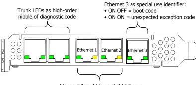
Ethernet 1 and Ethernet 2 LEDs as low-order nibble of diagnostic code
