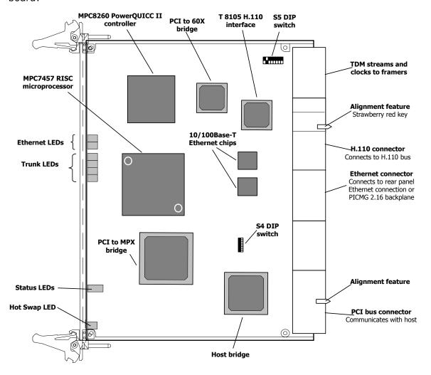
The following illustration shows the location of the main components on the rear I/O transition board. The transition board is attached to the TX 4000C board and enables the board to support the T1, E1, and Ethernet functionality.
