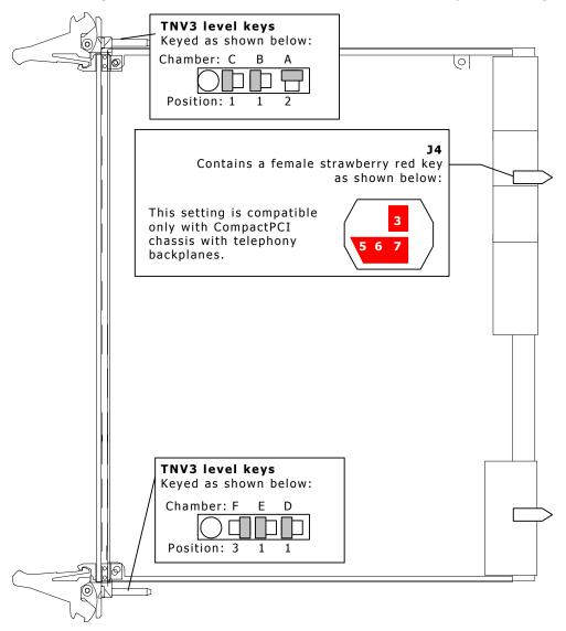
The following illustration shows some of the keying chambers in a CompactPCI chassis that you must configure for a TX 4000C. You must also key rear keying chambers A through F that are not shown.
