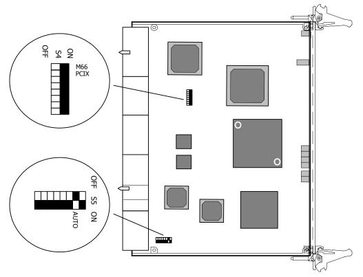
DIP switch S4 enables you to hot swap the TX 4000C into an older CompactPCI chassis. By default, the eight switches of DIP switch S4 are set to the OFF position. For normal board operations, do not modify any of the S4 switch settings.
