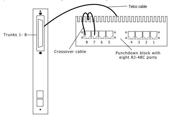
The crossover cable connects the transmit signals from one trunk to the receive signals on another trunk as shown in the illustration.
