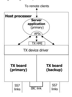
A single-node redundant signaling subsystem can survive both signaling link and board failures without a service outage. In addition, one board can be taken out of service at a time for upgrade or reconfiguration without impacting the service provided by the application.
