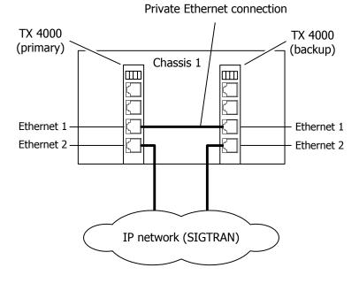
The following illustration shows a single-node redundant signaling server for TX 4000C boards:
