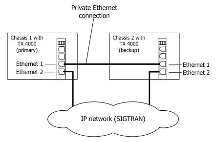
The following illustration shows a dual-node redundant signaling server for TX 4000C boards:
