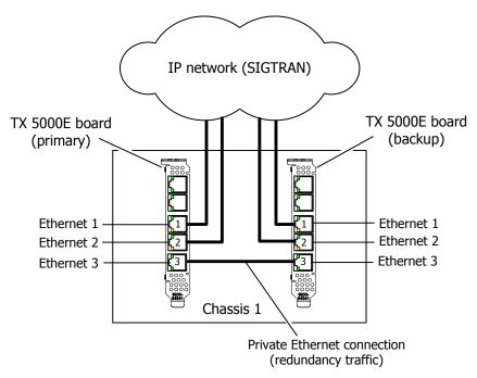
The following illustration shows how to set up two TX 4000 or TX 4000C boards based on a single-node signaling server in an IP network configuration. The boards are located in the same chassis to ensure board-level redundancy.
