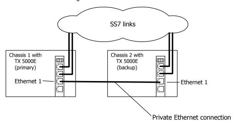
The following illustrations show how to set up two TX 4000 or TX 4000C boards based on a dual-node redundant signaling server in a TDM configuration. The boards are located in two separate chassis to ensure board-level and system-level redundancy.
