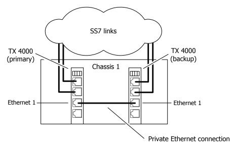
The following illustration shows a single-node redundant signaling server for TX 4000C boards:
