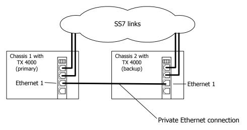
The following illustration shows a dual-node redundant signaling server for TX 4000C boards:
